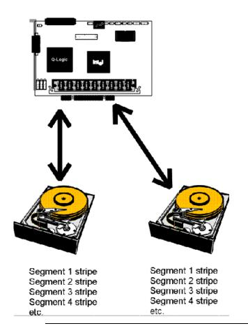
In RAID 1, MegaRAID Express 500 duplicates all data from one drive to a second drive. RAID 1 provides complete data redundancy, but at the cost of doubling the required data storage capacity.
